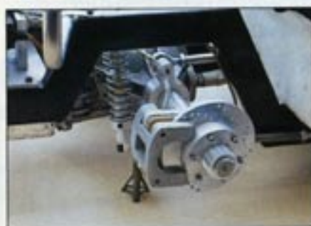
Cobra front A-arm suspension features adjustable shocks. Aluminum brake caliper grips with fiberglass pads (upper left). Rear suspension is 4-link setup. Rear disc brakes also are hydraulically activated (lower left). Cobra chassis shows fuel filler and dual master cylinders on rear platform (above).
